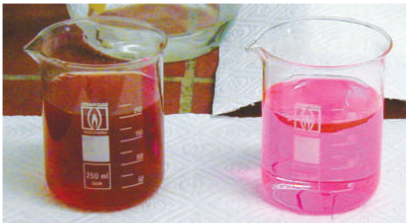
Fig 43. The effect of stagnation on Tyfocor solution
