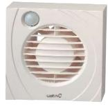
• Fitted with infra-red sensor activated by presence. • Timer (electronic timer adjustable from 3 to 15 minutes). • White finishing. · Plastic housing and impeller. • 230 V, 50 Hz motor, protection IP-X4, insulation class **B** as thermal cut out, ambient temperature SHO max. 40°C.
